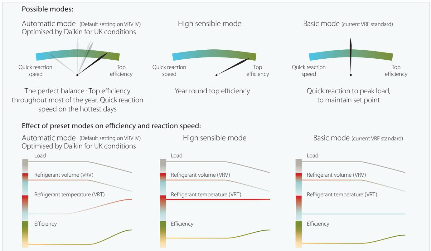
Revolutionary Variable Refrigerant Temperature (VRT) controls automatically adapt the VRV system to your individual building and climate requirements, thus drastically reducing operational running costs.
